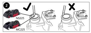
2 Pierce the middle of the protective cap on long guide sleeve using a suitable tool. Do not drive the tool between caliper bore and cap, as this might damage the caliper bore.
